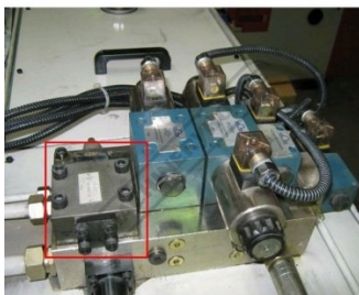
4HS9507 PILOT CHECK VALVE.2
