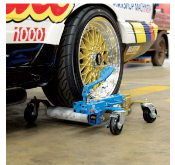
Wheel Jacked Ready to Move Vehicle
