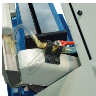
Coolant Shut Off Valve
