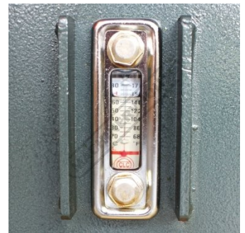
Hydraulic Oil Level Gauge
