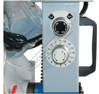
Adjustable Hydraulic Down Feed Control
