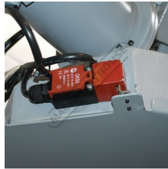
Safety Blade Guard Micro Switch
