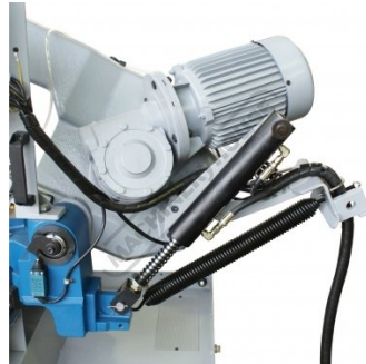
Motor and Gearbox Drive
