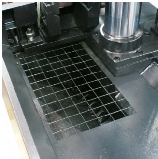
Chip Conveyor System
