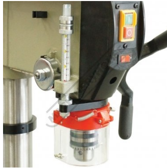
Drilling Depth Stop Setting with Scale
