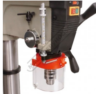
Drilling Depth Stop Setting with Scale
