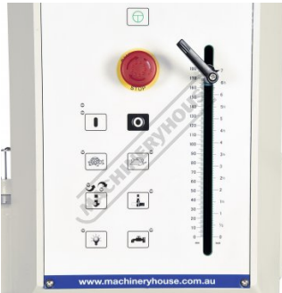
Depth Gauge And Control Panel
