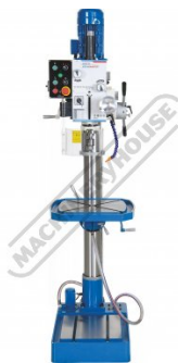
Adjustable Cast Iron table With T Slots
