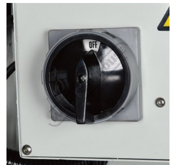
Main Isolation Switch
