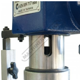
Drill Chuck Set Up For Removal
