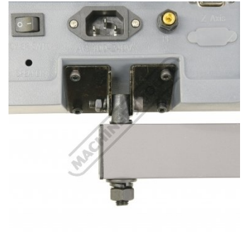
Mounting Close Up with Optional DRO
