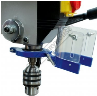
Safety Chuck Guard Flipped Up
