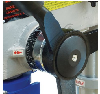
Drilling Depth Stop Setting With Scale
