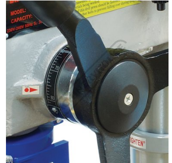
Drilling Depth Stop Setting With Scale
