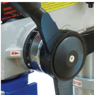
Drilling Depth Stop Setting With Scale
