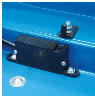
Safety Micro Switch on Pulley Guard
