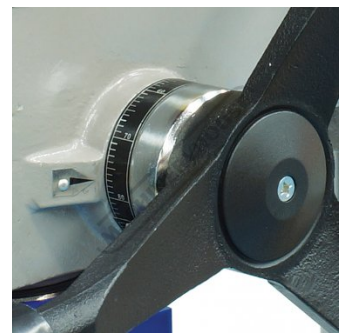
Drilling Depth Stop Setting With Scale
