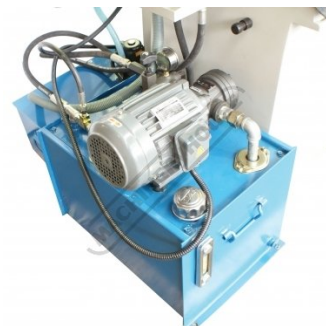
Hydraulic Unit & Coolant Tank
