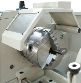
Chuck Guard With Safety Micro Switch
