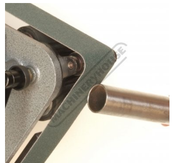
External Pipe Chamfering
