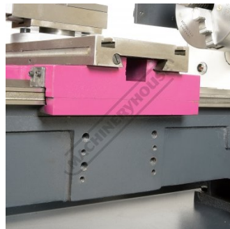
Mounting Point for Optional Milling Head
