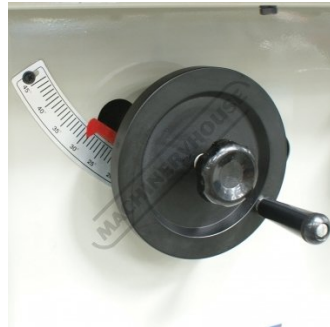
Blade Height Adjustment Handle & Angle Scale
