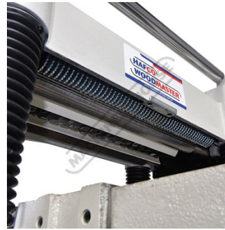
Six Spiral Cutter Head with 130 Inserts
