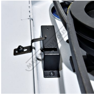
Safety Micro Switch on Belt Cover
