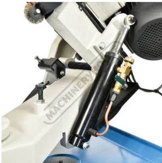
Hydraulic Ram Down Feed Control
