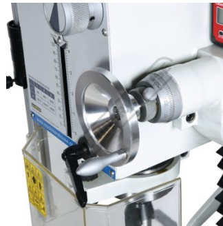
Fine Quill Feed Handwheel
