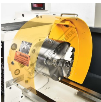
Chuck Guard with Safety Micro Switch
