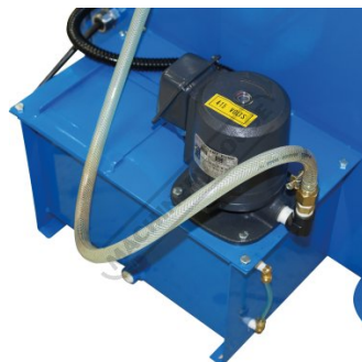
Coolant Pump and Tank
