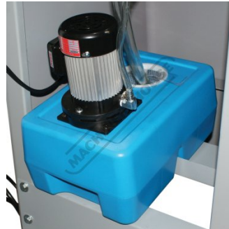
Coolant Pump and Tank
