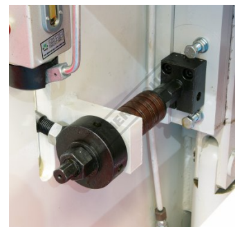
Quick Action Blade Clearance Adjustment
