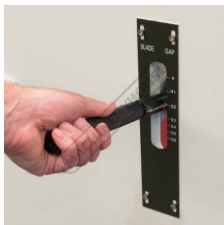
Quick Action Blade Clearance Adjustment Operation
