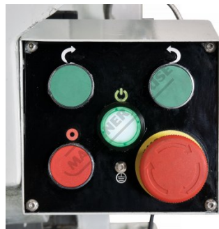
Horizontal Spindle Control Panel
