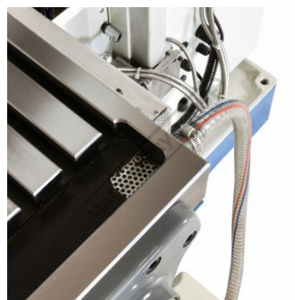
Work Table Coolant Return
