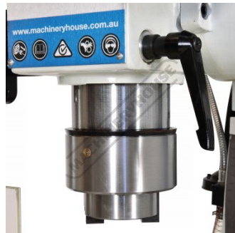
Vertical Spindle With Quill Lock
