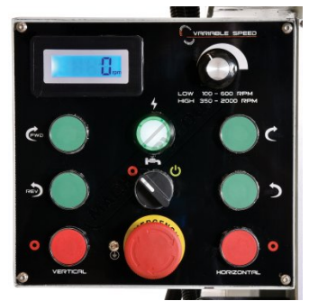
Control Panel With Digital Speed Readout
