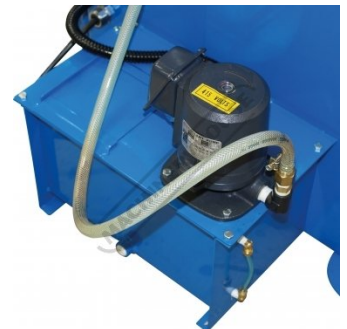
Coolant Pump and Tank
