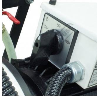
Main Power Switch
