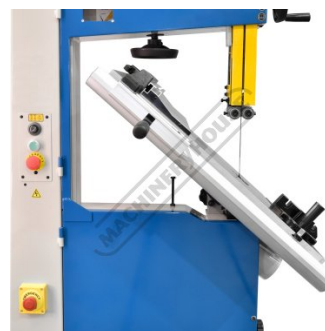
Cast Iron Table Tilts to 45 Degrees
