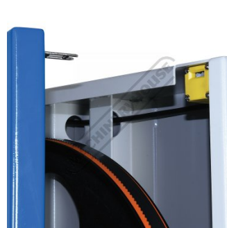
Safety Micro Switch On Door
