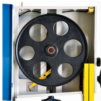
Cast Iron Blade Wheels
