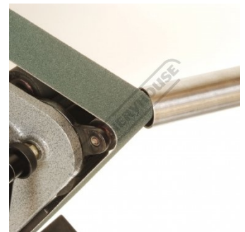
Internal Pipe Chamfering
