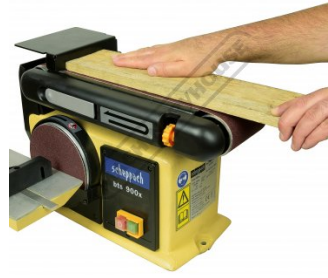
Shown Horizontal Flat Sanding
