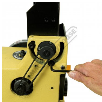
Lock / Unlocking Linishing Head Step 2 - Tighten Or Loosen 2x Cap Screws
