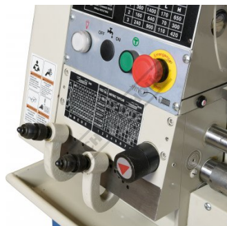
Feed Threading Levers and Control Panel
