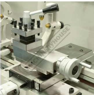
Compound Slide with 4-Way Toolpost
