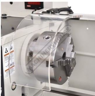
Safety Chuck Guard
