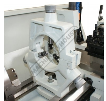
Fixed & travelling steadies with roller bearings
