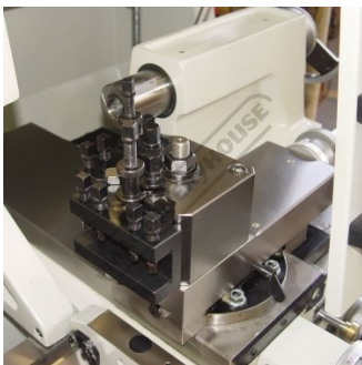
Quick change toolpost with additional holders
