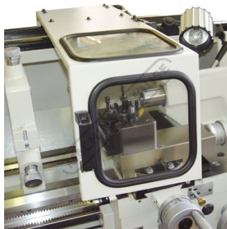
Sliding toolpost guard deflects swarf into tray
