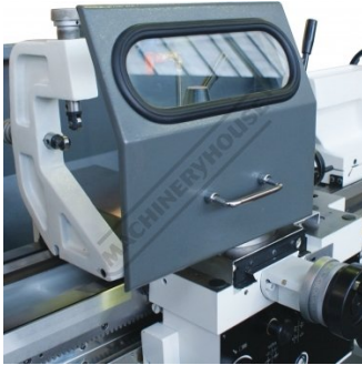
Sliding toolpost guard deflects swarf into tray-Closed
