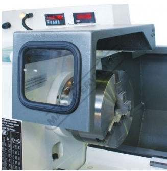
Chuck guard with safety micro switch cut out
