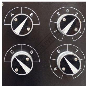
Gearbox Feed Controls
