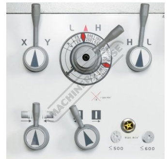
Speed Selections Levers and Feed Levers
