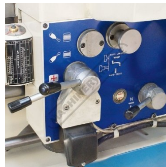
Saddle Feed Controls
