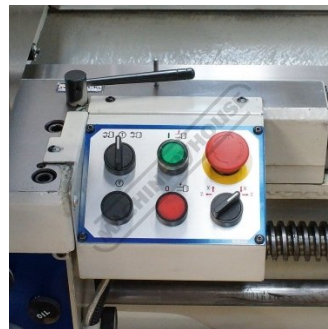
Saddle Switch Board
