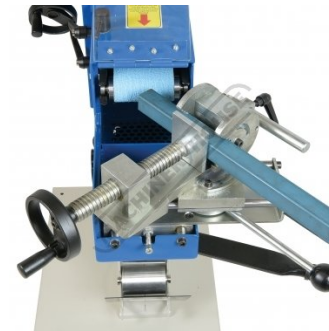
Square Vice Jaws Holding Material at 45 Degrees
