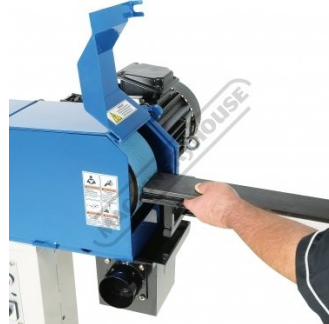
End Station Shown Linishing Flat Bar
