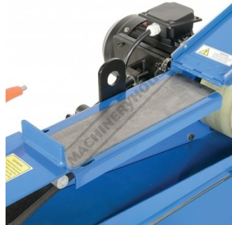
Top Station Includes Graphite Pad to Reduce Friction
