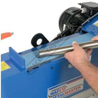
Top Station for Flat Linishing & Deburring
