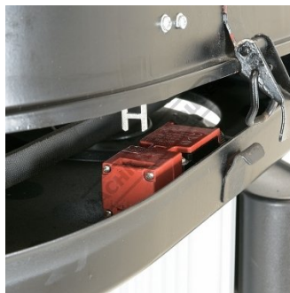
Safety Micro Switch on Belt Guard
