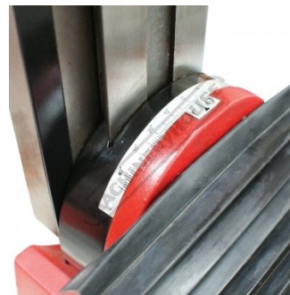
Milling head Tilts 45 Degrees both directions
